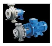
Centrifugal magnetically coupled (seal less) pumps are available in various material of construction. These pumps can deliver up to 550M3/Hr flow & 160M head. It can handle liquid up to 300 deg. c. temperature.
